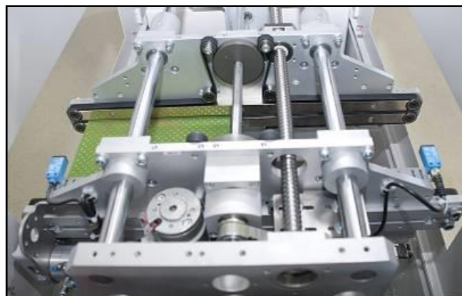
Flip axis in 180° position (stopper on the left side, closed)
