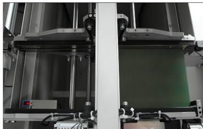
Flip axis in 0° position (stopper on the right side, closed)
