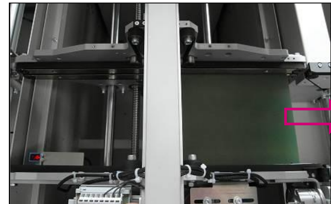
Stopper opens. Handover PCB to n+1
