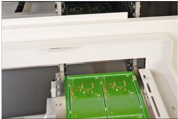
Buffer in take over position Take over the PCB from n-1
